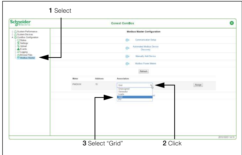
Figure 3-3 Power Meter Configuration
